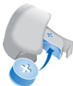
A magnet in the battery compartment ensures that the battery snaps noticeably into place.
